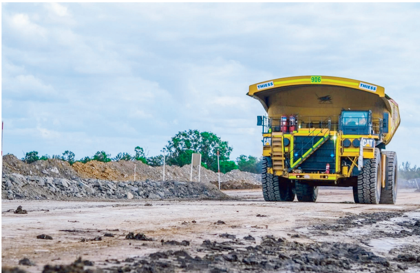
Thiess is trialling CNG on two of its mining fleet via a virtual gas pipeline from Rolleston to the Curragh coal mine near Blackwater.
